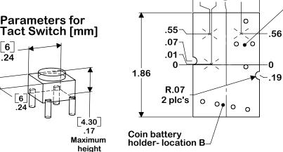
**Circuit Board** (.062" or .031")thickness overall dimensions (detailed drawing available)
