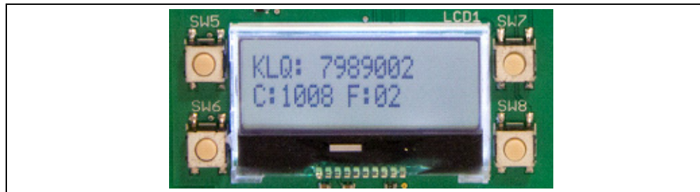
FIGURE 2-5: TYPICAL CLASSIC KEELOQ® TRANSMISSION
