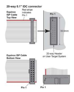
The **CAB-ARM-20W** cable is a **20-way** In-System Programming (ISP) ribbon cable designed to connect from any ISP programmer which features a 20-way IDC connector to a 20-way 0.1" pitch IDC connector on a suitable ARM microcontroller Target System. The cable features 200mm of flat ribbon cable with a 20-way 0.1" pitch female IDC connector on each end. The IDC connectors are fitted with 'cable grips' and are bump polarised to prevent the connector being plugged in the wrong way around.
