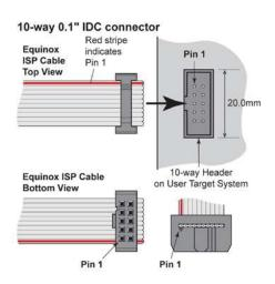
The **CAB-ISP10W200** is a **10-way** In-System Programming (ISP) ribbon cable designed to connect from any ISP programmer which features a 10-way IDC connector to a 10-way 0.1" pitch IDC connector on a suitable Target System. The cable features 200mm of flat ribbon cable with a 10-way IDC 0.1" pitch female connector on each end. The IDC connectors are fitted with 'cable grips' and are bump polarised to prevent the connector being plugged in the wrong way around.
