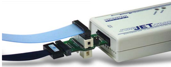
FIGURE 38 The JTAG-ETM splitter board attached to the JTAGjet-Trace emulator. Connected to it are a 20-pin ARM JTAG cable and an ETM Mictor cable (lower). A receptacle for an additional 14-pin TMS320 DSP JTAG cable is located at the bottom of the board.
