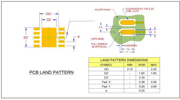
Figure 3 10-Pin DFN 3mm x 3mm PCB Footprint
