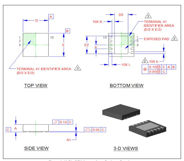
Figure 1 10-Pin DFN 3mm x 3mm Package Drawings
