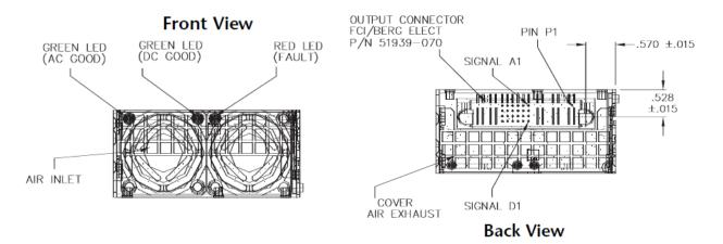
Input: 90V<sub>AC</sub> to 264V<sub>AC</sub>; Output: 48V<sub>DC</sub> @ 1200W; 5 V<sub>DC</sub> @ 0.5A
