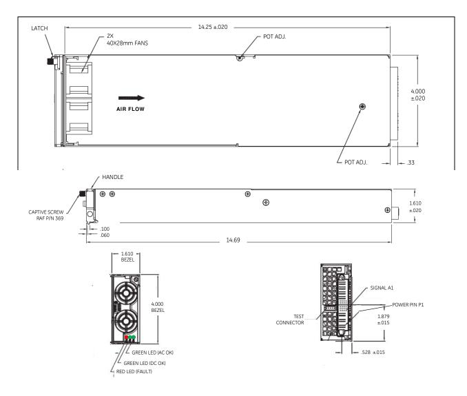
Input: 90Vac to 264Vac; Output: 48Vdc @ 2500W; 3.3Vdc or 5 Vdc @ 1A
