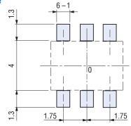
Note) The zero point is the center of mounting.
