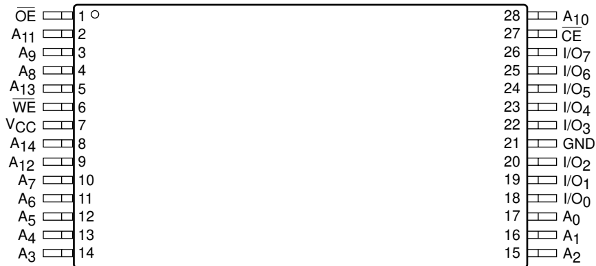
TSOP Top View (8mm X 13.4mm) (H)
