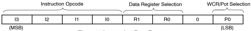
Figure 5. Instruction Byte Format
