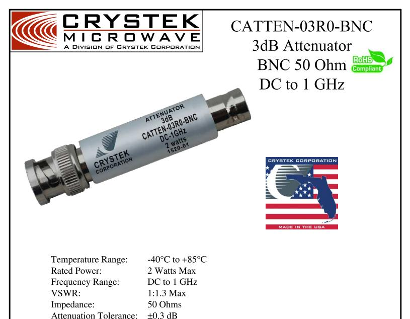
The Attenuator offers end users a rugged BNC attenuator housing for easy connection. The CATTEN-03R0-BNC provides 2 Watts of power dissipation. Tolerance matching is used to provide superior temperature tracking to individual components. Attenuator frequency range is from DC to 1 GHz.
