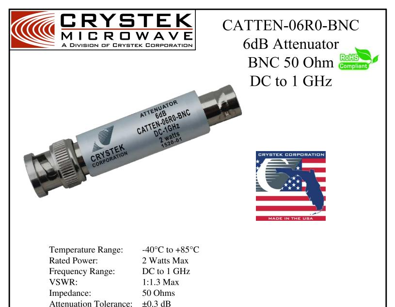
The Attenuator offers end users a rugged BNC attenuator housing for easy connection. The CATTEN-06R0-BNC provides 2 Watts of power dissipation. Tolerance matching is used to provide superior temperature tracking to individual components. Attenuator frequency range is from DC to 1 GHz.
