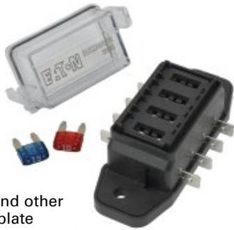
Mounting requires two customer-supplied #10 screws. Electrical connection is easily made with readily available, customer supplied 1/4" quick-connect terminals and 12 to 16 AWG\* wire.
