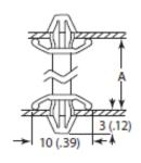
TO SNAP LOCK IN A 4 (.156) Ø HOLE, IN A 1.6 (.062) PANEL THICKNESS
