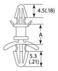
TO SNAP LOCK IN A 4.8 (.187) Ø HOLE, IN A 0.8 - 2.2 (.031 - .087) PANEL THICKNESS
