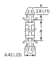
TO SNAP LOCK IN A 3 (.118) Ø HOLE, IN A 1.2 - 2 (.047 - .078) PANEL THICKNESS
