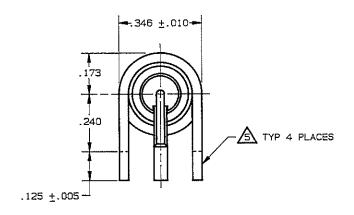
PRE-TINNED, .0015 MAXIMUM THICKNESS WITH SN63 OR EQUIV SOLDER, PER QQ-S-571, TO WITHIN .060 MAXIMUM OF SHOULDER, AFTER PLATING
