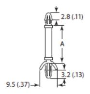
TO SNAP LOCK IN A 3 (.118) Ø HOLE, IN A 0.8 - 2 (.031 - .078) PANEL THICKNESS
