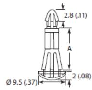
TO SNAP LOCK IN A 5.5 (.216) Ø HOLE, IN A 0.8 - 1.6 (.031 - .062) PANEL THICKNESS
