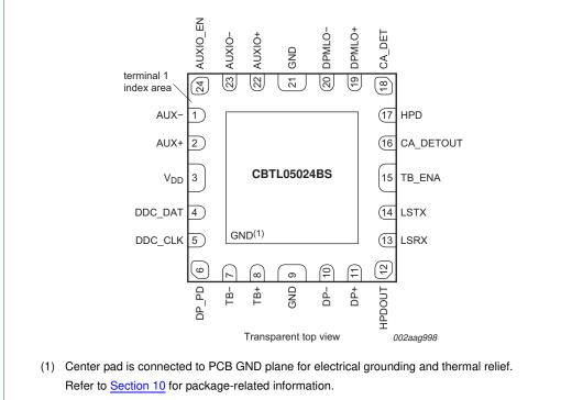
Fig 2. Pin configuration
