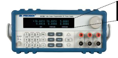
The 9130 is a fully programmable triple Output DC Power Supply delivering 0-30V/0-3A on 2 outputs and 0-5V/0-3A on 1 output. Each output is fully floating and outputs can be adjusted independently or connected in series or parallel to produce higher voltages or currents. The 9130 is ideally suited for applications in Electronic Test, Production and Service where multiple independent DC supplies are required and bench space is at a premium.
