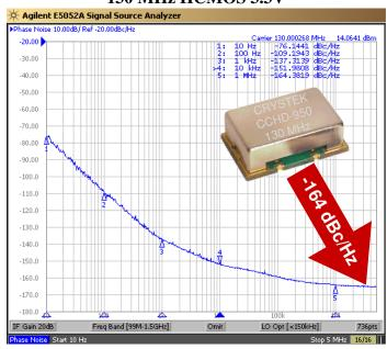
Model CCHD-950 is a 45 MHz to 130 MHz HCMOS Clock Oscillator. High Q crystal and 3<sup>rd</sup> overtone technology provides Ultra-Low Phase Noise and Low-Jitter performance with an HCMOS output. Features include -165 dBc/Hz phase noise floor with 3.3 Vdc input voltage, -40°C to +85°C operating temperature, and 9×14 mm SMT package. The oscillator has no sub-harmonics. Rev: K
