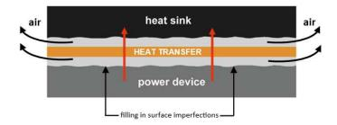
Note: during initial phase-change, it is recommended to re-check your torque settings if device utilizes a screw mounting system. Applying additional torque during initial phase change will thin the material bond line slightly leading to improved thermal performance.
