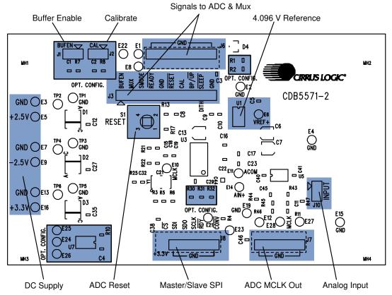
NOTE: Shaded boxes marked with "OPT. CONFIG." are not necessary for operation in an end user product.
