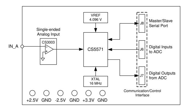
Figure 1. CDB5571-2 Block Diagram
