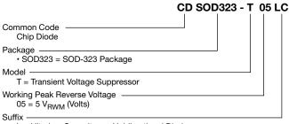
L = Ultralow Capacitance Unidirectional Diode LC = Ultralow Capacitance Bidirectional Diode
