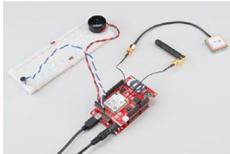
Full-size breadboards are perfect for creating a breadboard handset.
