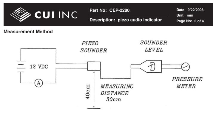
S.P.L. Measuring Circuit Mic: RION S.P.L. meter UC 30 or equivalent S.G.: Hewlett Packard 33120A Function Generator or equivalent
