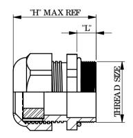
NO TES: TEMPERATURE RANGE -20 °C TO +100 °C PROTECTION GRADE IP68 - 5 BAR
