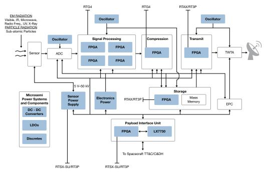
RTSX-SU, RTAX, and RT ProASIC3 FPGAs are used for command, control, and interfacing applications, where limited logic and performance is needed. RTG4 can be deployed where maximum data throughput is needed, such as in signal processing and compression.
