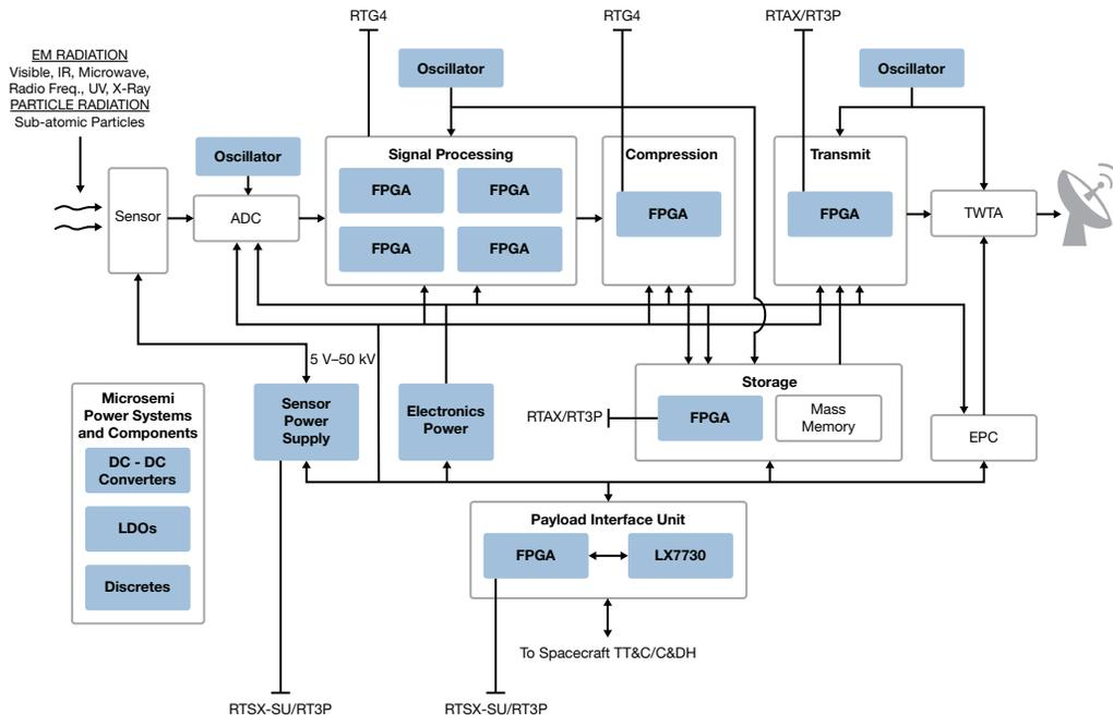
RTSX-SU, RTAX, and RT ProASIC3 FPGAs are used for command, control, and interfacing applications, where limited logic and performance is needed. RTG4 can be deployed where maximum data throughput is needed, such as in signal processing and compression.
