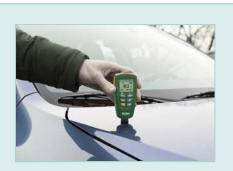
Measuring the thickness of automotive paint
