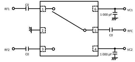
Note C0 : 0.05 to 0.5 GHz 1,000pF : 0.4 to 2.0 GHz 56pF : 2.0 to 6.0 GHz 8pF
