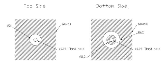
\*The antenna feeding in transmission line should connect with the  $\varphi$  2.5 circle at the Bottom Side, and keep transmission line impedance at 50 ohms for good power transmit from system to antenna.
