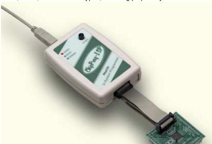
The programmer has three LEDs for displaying the programming status ("Good", "Busy", "Error") and the "Start" button for fast launch of the pre-programmed command chains. The tool shown on the picture is very small and requires no power adapter for the operations - it gets power from the USB computer port.
