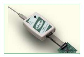
The <u>ChipProg-ISP</u> is a low-cost device programmer for engineering, field service and manufacturing. Unlimited number of these device programmers can be driven from one PC and can run concurrently to program multiple devices at a time. This device programmer works under control of the <u>ChipProgUSB</u> software pack.
