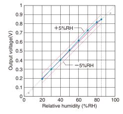
□EXAMPLE OF THERMAL CHARACTERISTICS (TEMPERATURE DEPENDENCY) at Edc=5V, +15 to +35°C, 20% to 85%RH
