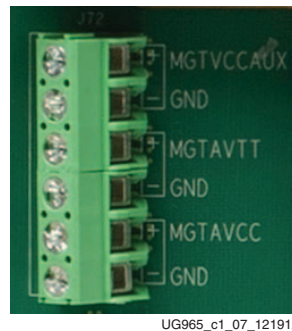
Figure 1-7: GTH Transceiver Power Terminal Block J72
