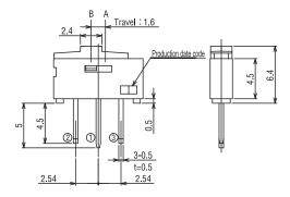
Unless otherwise specified, tolerance:  $\pm$  0.3 (Unit: mm)
