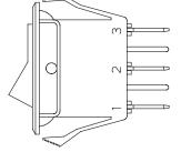
NOTE: Orientation of actuator marking and terminals.
