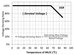
This product ,which guarantees High Temperature Reliability Test with 100% of rated voltage at the maximum temperature, recommended to be used in the circuit with derat is recommended to be used in the circuit with derated voltage compared to the rated voltage of the capacitor for long lifetime.
