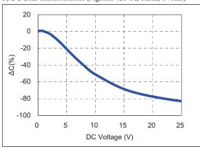
4) Bias TCC characteristics (Agilent 4284A, 1kHz, 1Vrms, 12.5Vdc)
