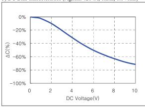
4) Bias TCC characteristics (Agilent 4284A, 1kHz,1.0Vrms,5Vdc)
