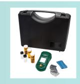
Meter comes complete with all the accessories to conveniently take measurements of both Free and Total Chlorine up to 3.50ppm with 0.01ppm resolution. The method used is adapted from USEPA Method 330.5 for waste water and Standard Method 4500-Cl-G for drinking water.
