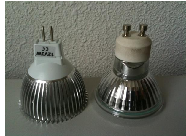
Two most common MR16 connectors • GU5.3 (left) for low voltage inputs • GU10 (right) for direct AC inputs.
