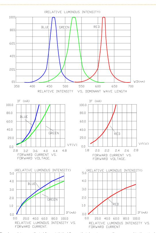
The above data are collected from statistical figures that do not necessarily correspond to the actual parameters of each single LED. Hence, these data will be changed without further notice.
