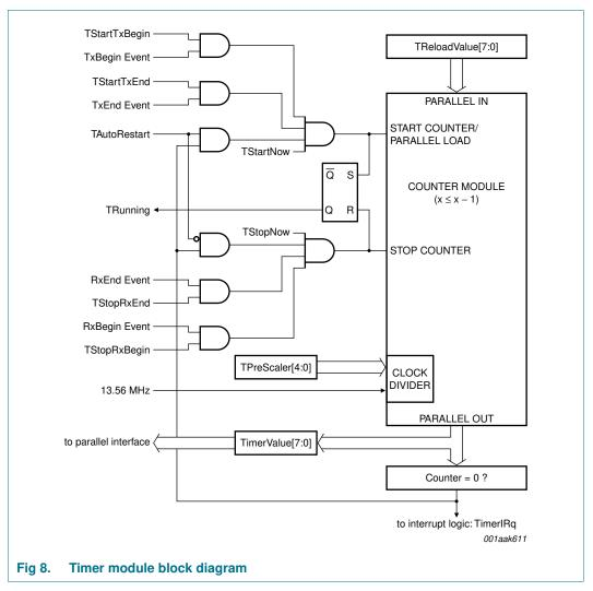
The timer unit is designed, so that events when combined with enabling flags start or stop the counter. For example, setting bit TStartTxBegin = logic 1 enables control of received data with the timer unit. In addition, the first received bit is indicated by the TxBegin event. This combination starts the counter at the defined TReloadValue[7:0].
