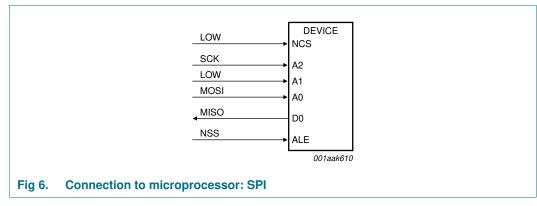
**Remark:** The SPI implementation for CLRC632 conforms to the SPI standard and ensures that the CLRC632 can only be addressed as a slave.
