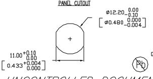
\*UNLESS DTHERWISE SPECIFIED TOLERANCES PER DECINAL PRECISION ARE: X=±1 (±0.039), X.X=±0.5 (±0.020), X.XX=±0.25 (±0.010), X.XXX=±0.127 (±0.005). LEAD SIZE=±0.05 (±0.002), LEAD LENGTH=±0.75 (±0.010). MIN= +DECINAL PRECISION MAX.= +0.00 MAX.= +0.00
