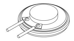
SPECIFICATIONS: WIRE: UL1007, #28AWG LENGTH: 152mm
