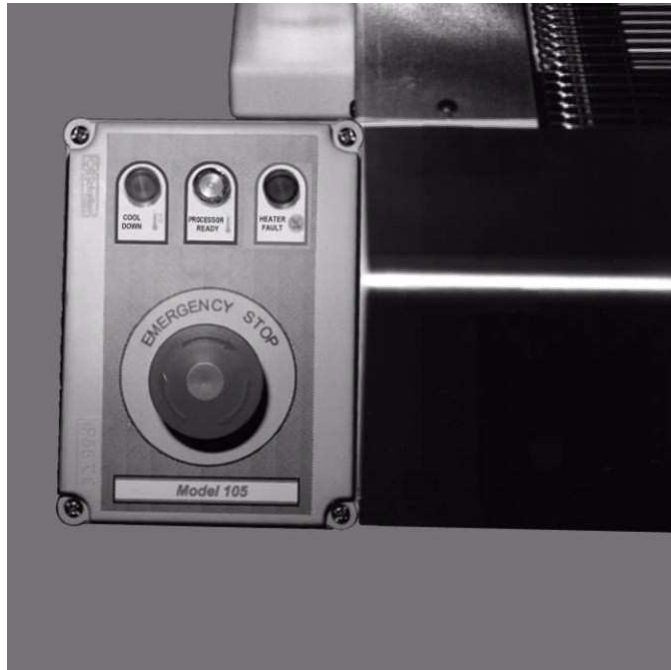
Emergency Stop Enclosure
