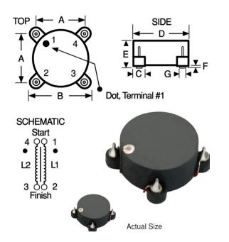
Mechanical Configuration A flat top surface mount case with excellent coplanarity of terminals.
