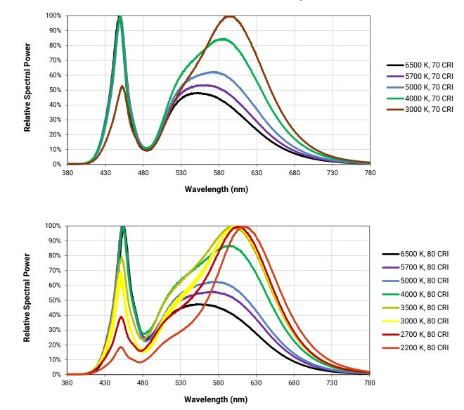
The following graphs are the result of a series of pulsed measurements at 1400 mA and  $T_1$  = 85 °C.
